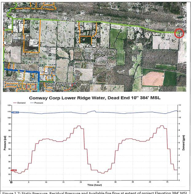
Figure 1.7: Static Pressure, Residual Pressure and Available fire flow at extent of project Elevation 384' MSL
